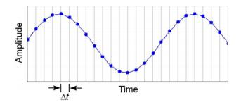
Figure 1.2: The sinusoidal curve represents the continuous analog waveform being sampled. Measurements of the instantaneous amplitude of the signal are taken at a sampling rate of  $\Delta t$  [ft].
